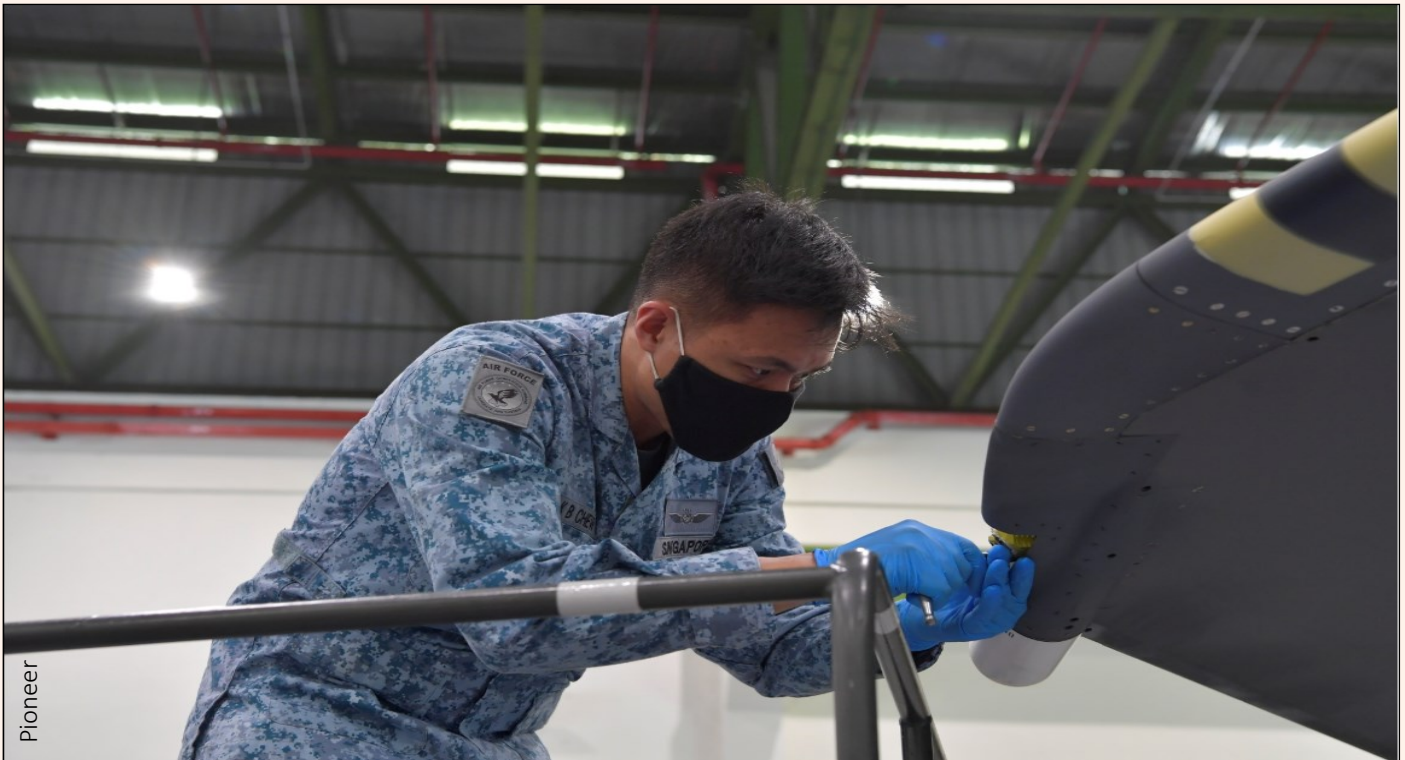
ME2 Benny Chew replacing the LED module in the wing position light of the F-15SG.
